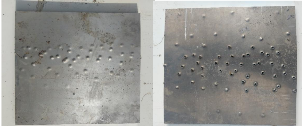
Figure 1; Images showing the rear face of the 12.7mm (L) and 8mm (R) test plates for DTG-5 qualification as defined in PAS-300. No penetrations of the thicker panel and >50% penetration of the thinner panel as required in the standard performance criteria.
