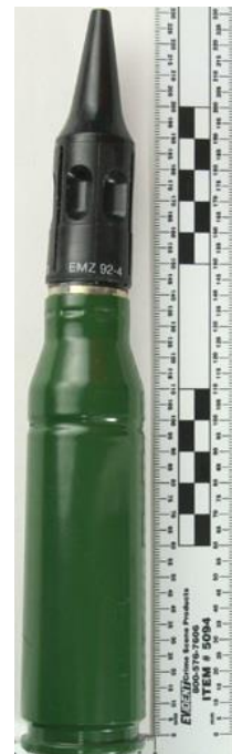
Figure 2 (right); Complete, 25x137mm APDS-T round
