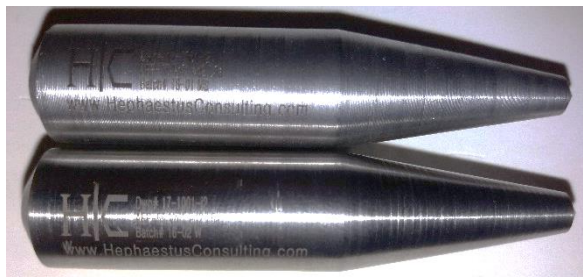
Figure 1 (left); Complete Hephaestus Surrogates, 25x137mm APDS-T flight surrogate (top) and full (bottom)
